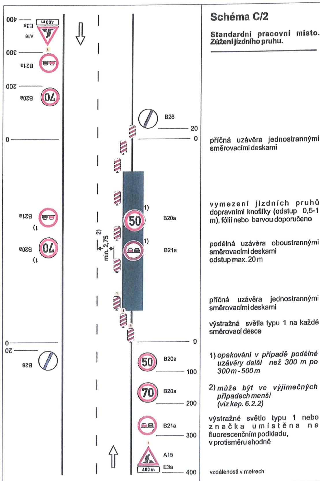
**SCHÉMA PDZ PŘI POUŽITÍ SEMAFOROVÉ SOUPRAVY, UZAVŘENÍ
